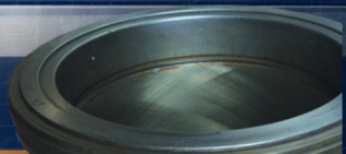
AFTER HONING PROCEDURE (MAGNIFICATION X 50)
